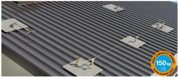
The Travflex™ 2 single-cable system provides a smooth travel. It allows the slider to move freely over the intermediate anchors, minimizing wear and eliminating user assistance. The user's hands remain free to accomplish whatever task is required. It is designed to limit the forces transmitted to the structure in the event of a fall for installation on light structures such as steel deck roof.
